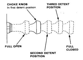
Fast idle should be: 1,500-2,500 min-1 (rpm)
