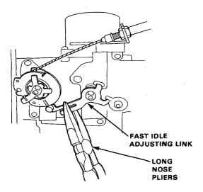
If the engine speed is too low, insert a screwdriver in the fast idle adjusting link slot and widen the slot.
