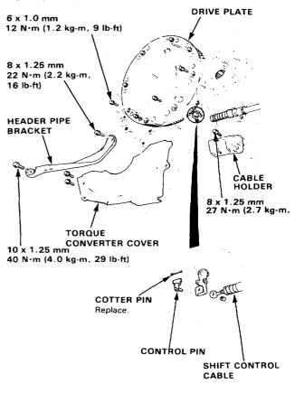
Install the torque converter cover and header pipe bracket.
